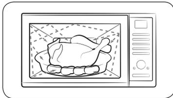
1. The microwaves generated by the magnetron reflected at cavity and are distributed uniformly as the food rotates on the turntable. The food is thus cooked evenly.
